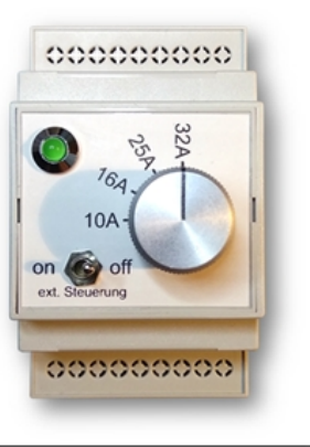
Picture 17: EVSE WB in custom box with 4position current switch
